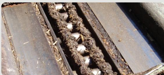
Regular and less lubrication is more effective than infrequent and too much. There must always be a sufficient amount of lubricant between pins, bushes and rollers (chain joints) to reduce wear, protect against corrosion and reduce operating noise.
